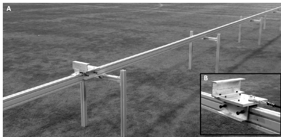
Fig. 1. Photograph of the 12 m monorail (A) with sliding platform (B) which was towed by the athlete during the 10 m sprints. Two GPS devices spaced 30 cm apart were secured to a bracket which was bolted to the platform.
